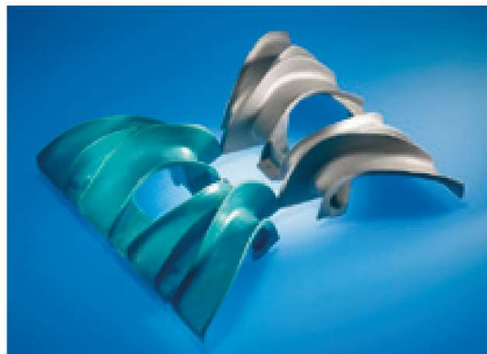
Indirect Manufacturing. Air intake manifold; AM master made from polystyrene by laser sintering after surface treatment (left), aluminum casting, one-of-a-kind part (right)
