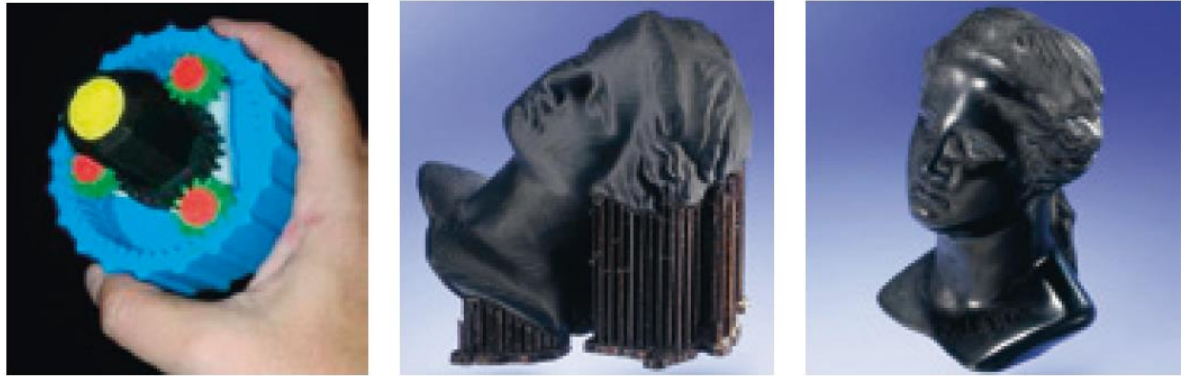
Figure 3.6 - Fused deposition modeling. Epicyclic gear set assembled from monochromatic FDM parts, made from ABS plastic (left); part with support as manufactured (center); part after removal of the supports and manual polishing (right)
