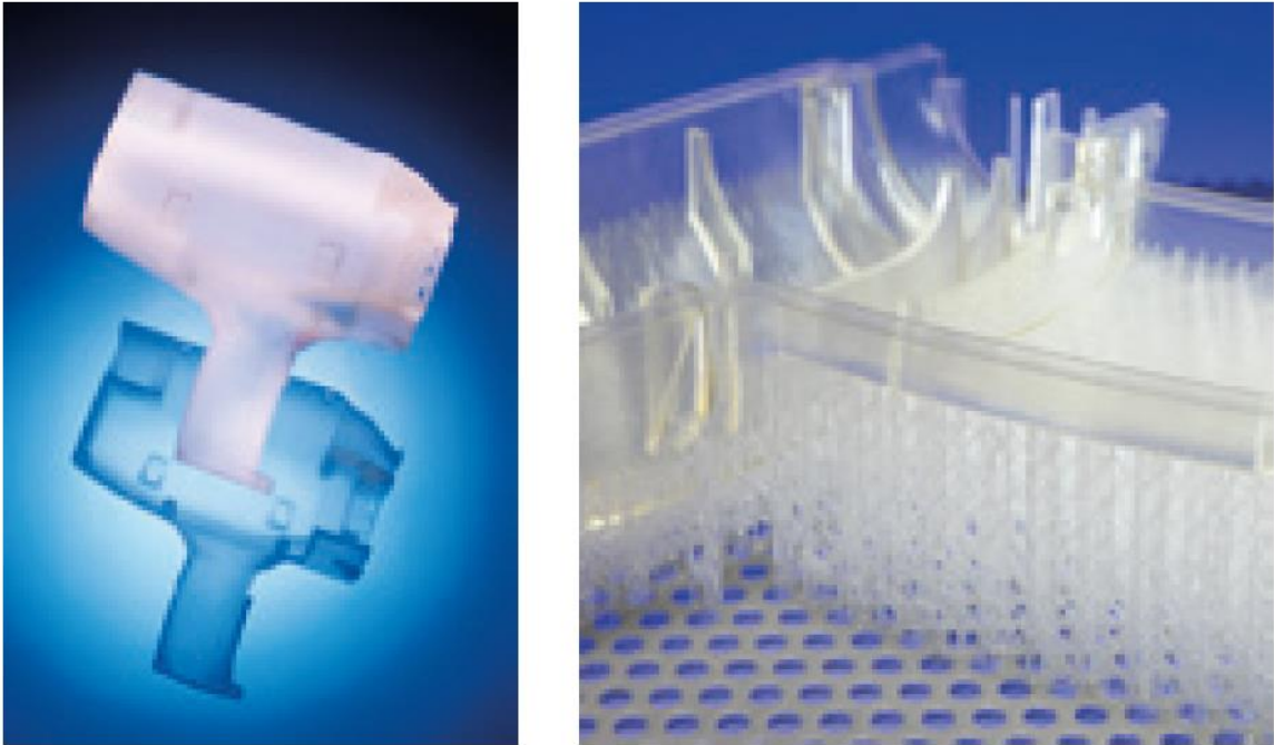
Figure 3.3 - Laser stereolithography; thin-walled shell type parts (left), part with supports on the build platform (right)
