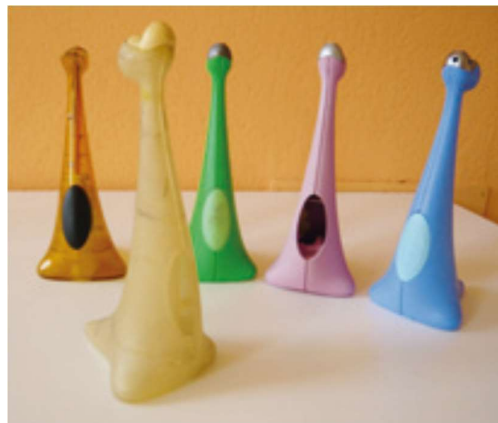
Indirect prototyping; silicon rubber molding; lighter “Bruce”; AM master, stereolithography; working RTV copies
