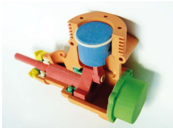
Solid image or concept model. Cut-away demonstrating part of a combustion engine unit; 3D-printing
