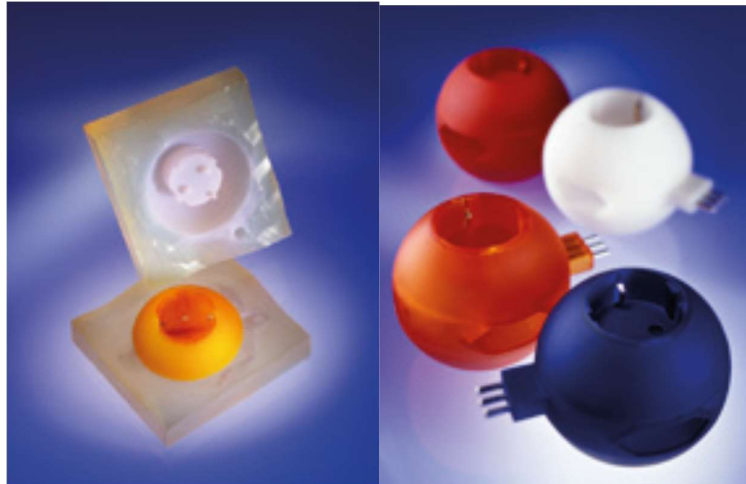
Indirect prototyping; silicon rubber molding; plug system; master made by stereolithography; mold with upper part of plug housing (left), mounted plugs (right)
