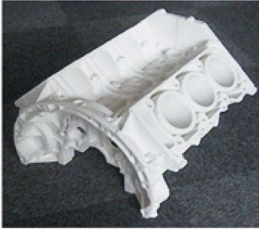
Indirect manufacturing; combustion engine housing; AM master (left), laser sintering, polystyrene; aluminum casting, one-of-a-kind part (right)
