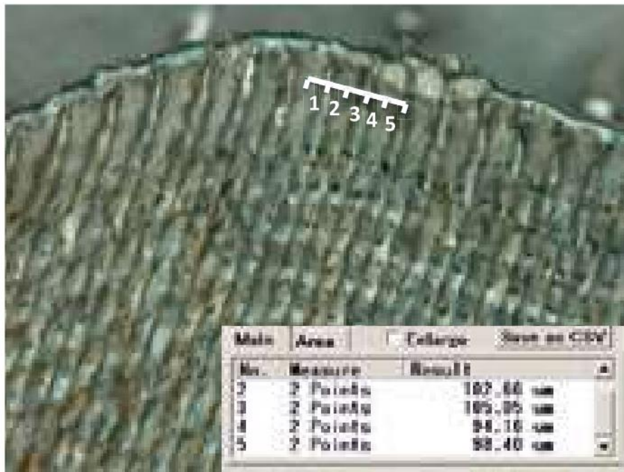
Figure 4.3 Top layer of a laser sintered metal part (SLM)
