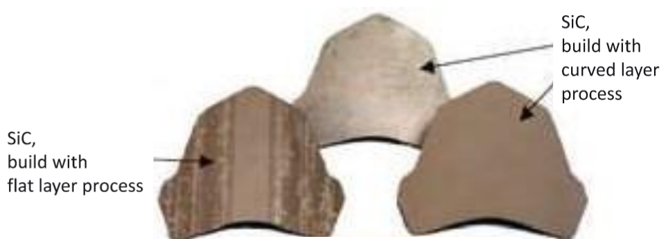
FIGURE 4.5 Layer laminate manufacturing (LLM); reinforced curved parts with integrated SiC fibers /Klo99/
